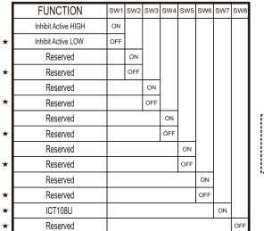
This dip switch is located on the CPU board, remove the CPU board cover first.
